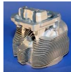
Figure 10: An air-cooled cylinder head cast in Al-Ce8 alloy
