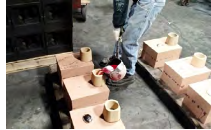
Figure 5: Pouring raw castings from hybrid composite material
