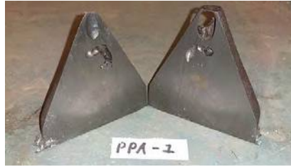
Figure 6. Example of solidification shrinkage in a cone specimen.
