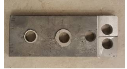
Figure 7. Locations of extracted specimens (pins) in plate casting (a) and extracted pin (b).
