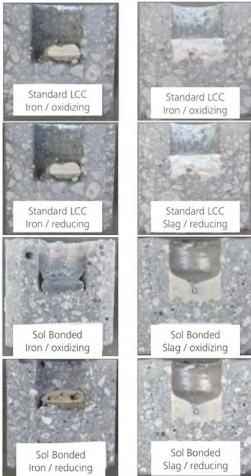
Figure 7. Images of slag cups sectioned after testing
