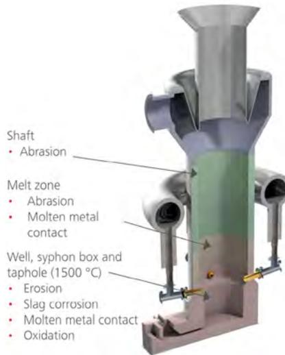
**Figure 1.** Typical lined Cupola (atmospheric front slagging)
