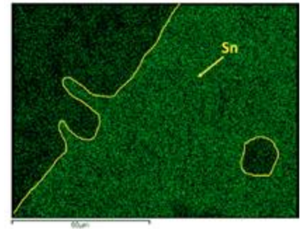
Fig 9. Examples of nonuniformity in the Cu and Sn distribution. a) Analyzed sample image, b) areas with increased Cu content, b) area with increased Sn content.
