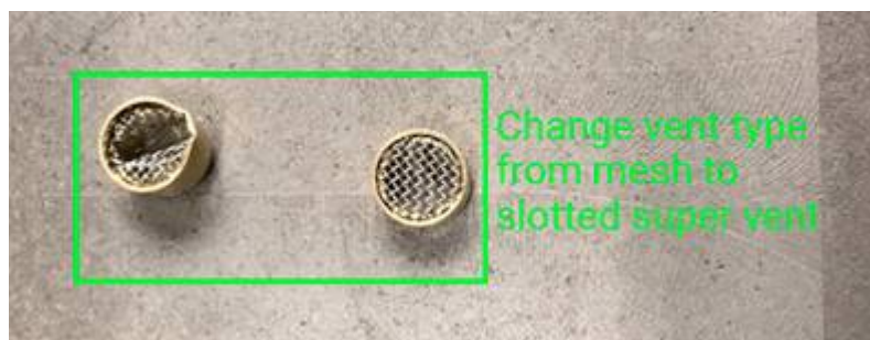
Pic 1 + 2: The ASKNow service visit helped to solve binder build-up and plugged-up tooling vents.
