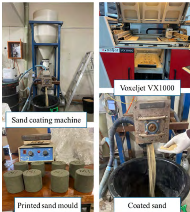
Laboratory equipment and materials used in this study included the sand coating machine, coated sand, printed sand moulds and 3D printer.
